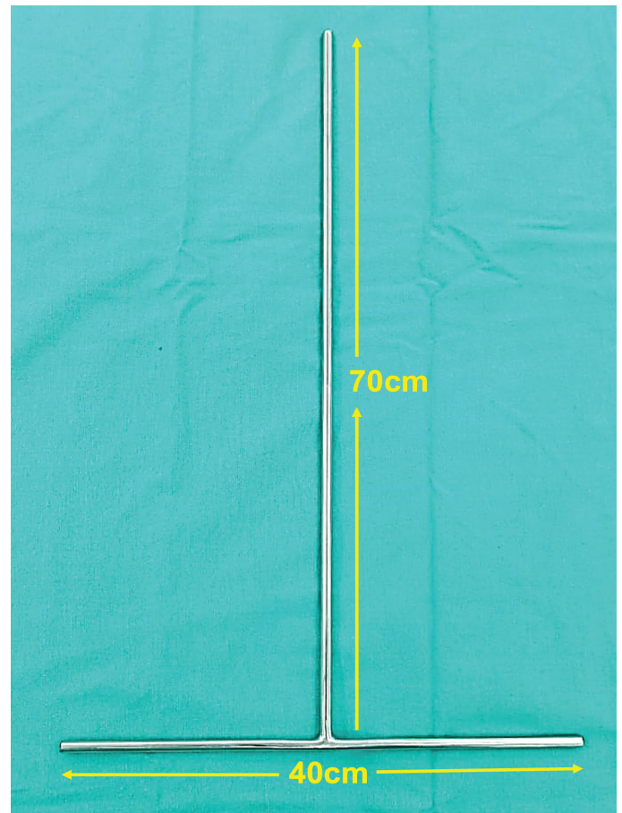
Figure 1. The horizontal arm of the T-tool is 40 cm and the vertical arm is 70 cm. The device is constructed with stainless steel
